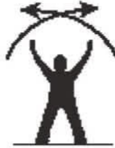
LZ unsafe (day)
