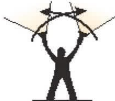
LZ unsafe (night)
