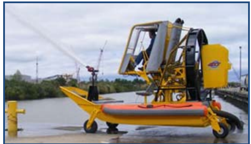
Figure 42. This innovative, amphibious emergency vehicle combines the versatility of an airboat with full fire-fighting, EMS, and rescue capabilities.
