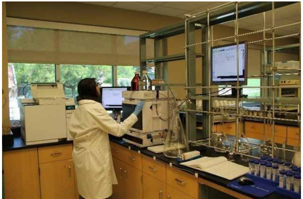
PhD candidate, Purni Wickramasinghe, isolating bioactive molecules from mushrooms using preparative-high performance liquid chromatography (prep-HPLC).
