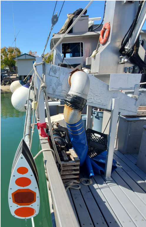
Figure 4: Transducers (Top-bottom: Simrad ES200-7C, ES120-7C, ES38-12, and ES70-7C, Kongsberg) in a pole-mounted multi-transducer array (MTA4) installed on the Long Beach Carnage .
