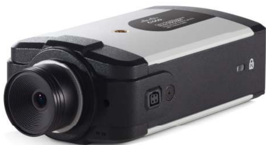
Figure 1. Cisco PVC2300 Business Internet Video Camera: Audio/PoE
