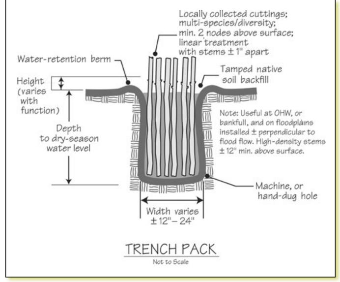
Figure 3–72—Installing trench packs (Eubanks and Meadows 2002). OHW stands for ordinary high water.
