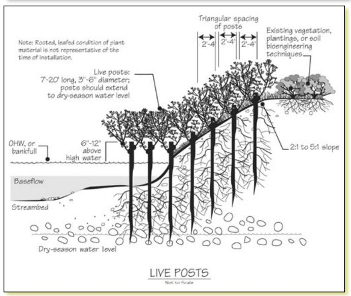
Figure 3–63—Live posts reduce stream velocities, allowing sediment to be deposited (Eubanks and Meadows 2002). *OHW* stands for ordinary high water.
