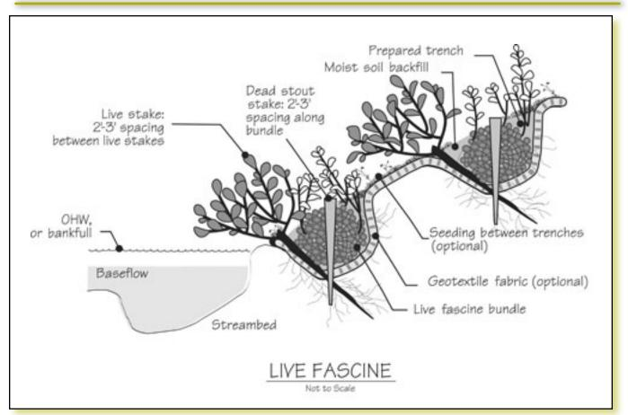
Figure 3-69a—Installing live fascines (Eubanks and Meadows 2002). OHW stands for ordinary high water.
