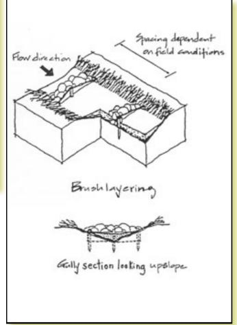
Figure 3–67—A gully can be treated with brush layering. Drawings courtesy of Lisa Lewis (Lewis and Ogg 1996).
