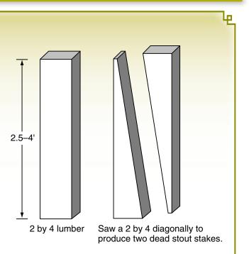
Figure 3–61—Dead stout stakes, cut from 2 by 4s (about 50 by 100 millimeters), are used in many soil bioengineering techniques to anchor branches or erosion control blankets, and to anchor erosion control blanket logs to the bank. (Eubanks and Meadows 2002).
