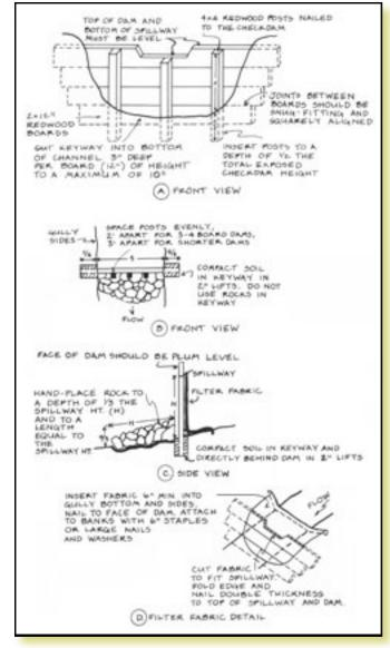
Figure 3–55a—Checkdam installation. Wooden checkdams are constructed by stacking logs or split rails. Drawings courtesy of Liza Prunuske (1987).
