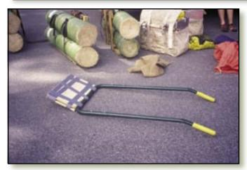
Figures 5–2—When transporting a U-bar digger using stock, cover the tool's sharp tines with a homemade scabbard.
