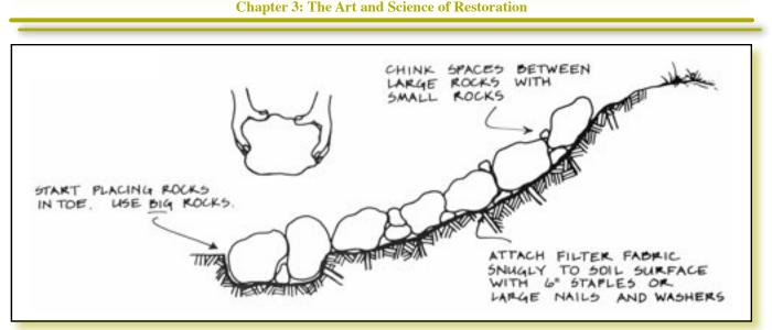
Figure 3-49-Placing rock for riprap. Drawings courtesy of Susan Pinkerton (Prunuske 1987).
