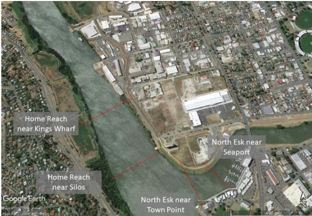
Figure 30. Location of cross sections used in analysis of North Esk tidal floodplain scenarios. Note there is no change in the tidal prism of the Yacht Basin so it is expected these options will not impact on cross-sections in that location.
