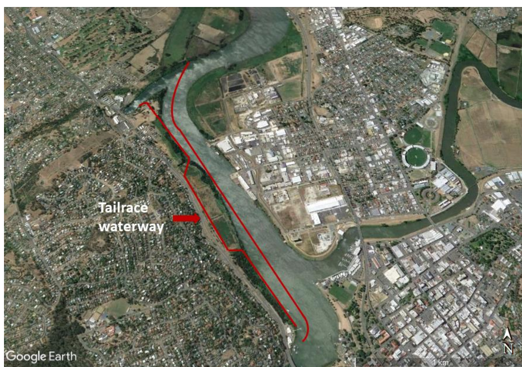
Figure 36. Proposed location of waterway to return Tailrace flows to upper estuary near Kings Bridge.
