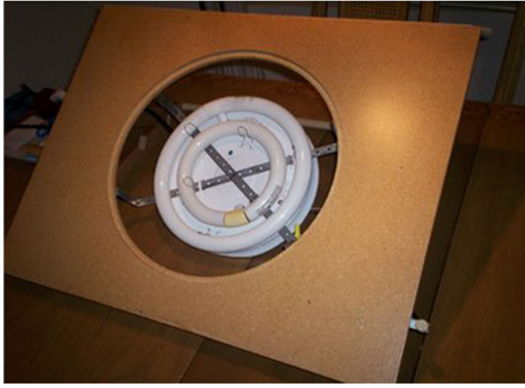
7) Back light unit attached.
