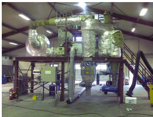
A variety of feedstocks have been torrefied at the test reactor: woodchips, grass, straw, palm oil kernels, etc.
