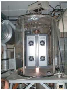
Special reactor design: 1-2s residence times with only limited total reactor length
