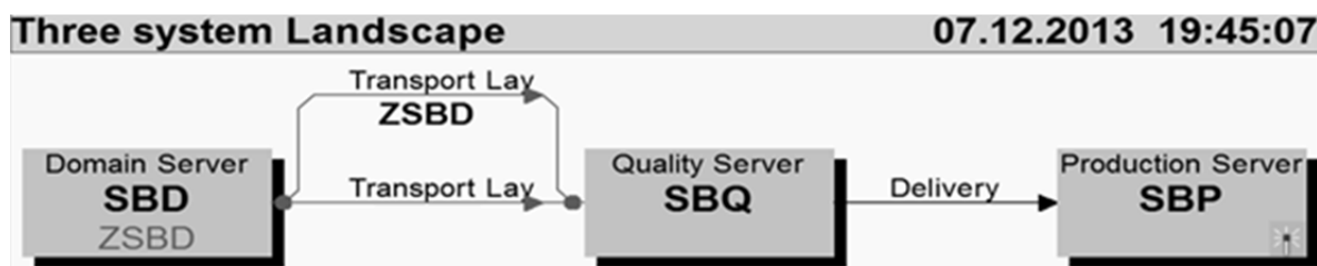
Fig 2.8.3: Three separate environment for development, testing and production
