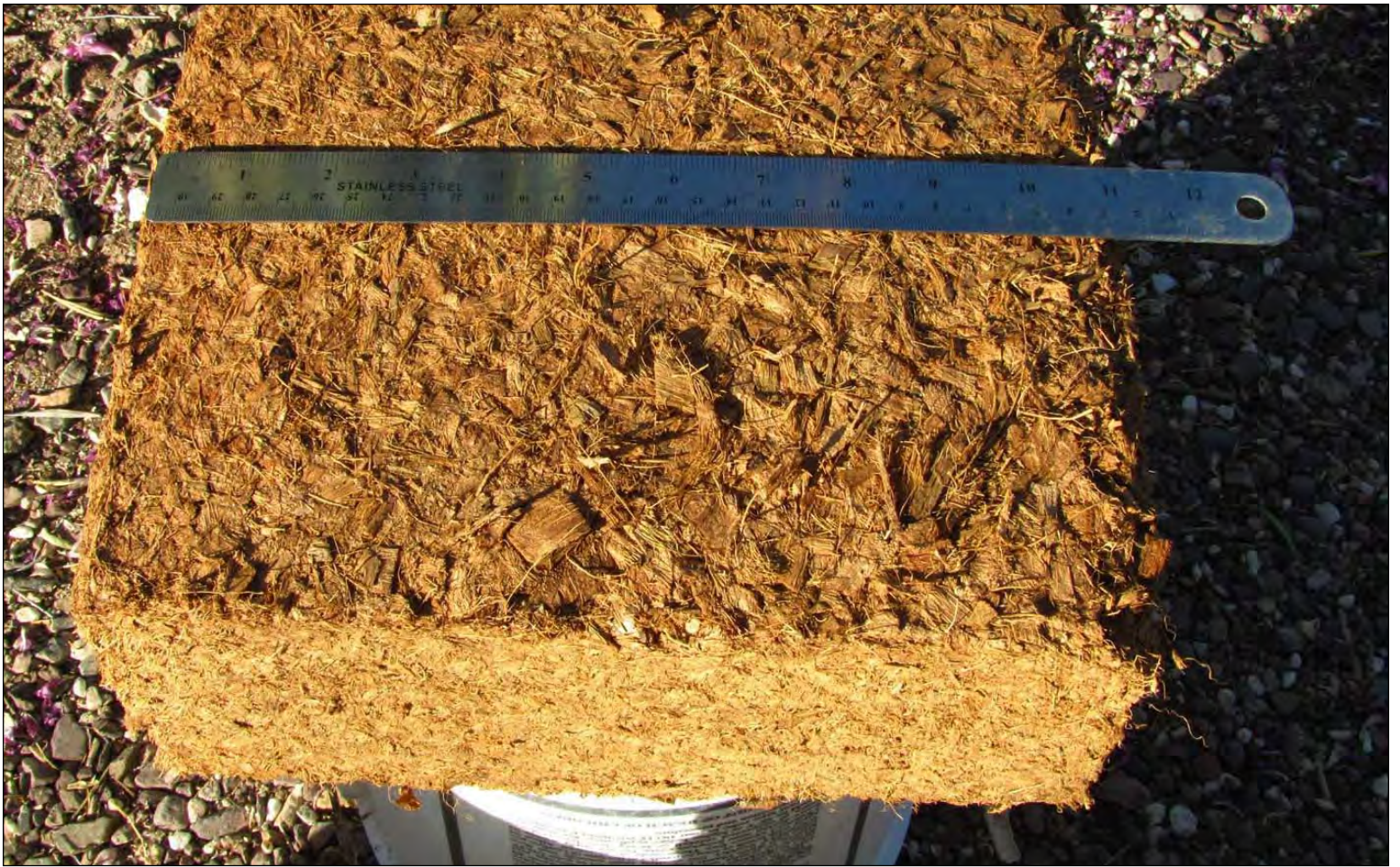
Figure 3. Coir is commonly sold as blocks of about a half cubic foot.
