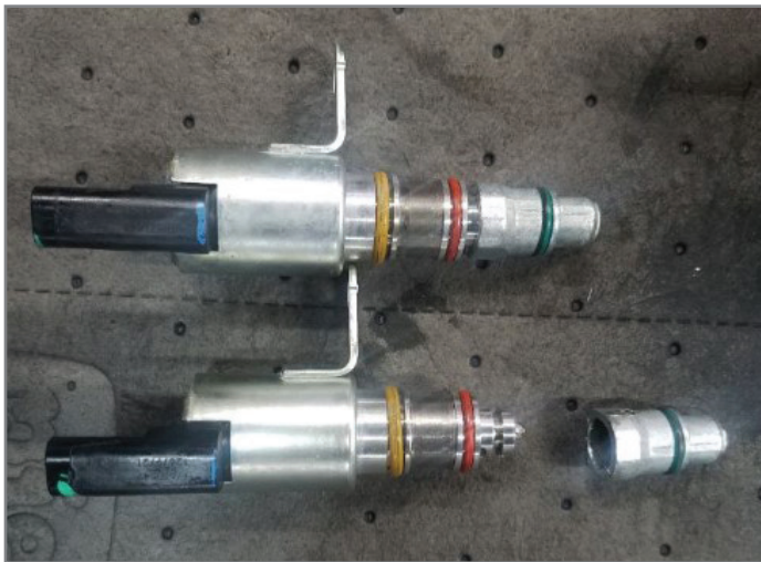
A complete solenoid, top, and a broken solenoid, bottom
