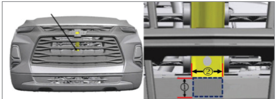
Trim the foam block and insert it between the close-out panel rear vertical wall and center fascia support bracket.
