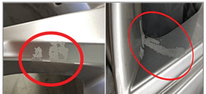
Paint run condition warrantable by refinishing.
