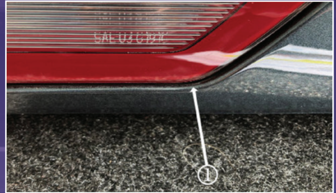
Interference at the CHMSL and body of the roof-mounted spoiler.
