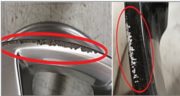
Damage from curb scrapes are not warrantable repairs.
