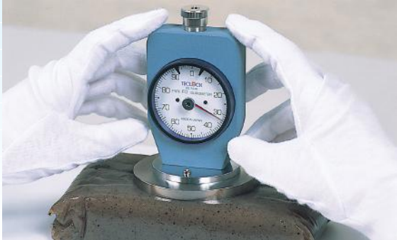
Hardness measurement of Konjac. Durometer : GS-744G
