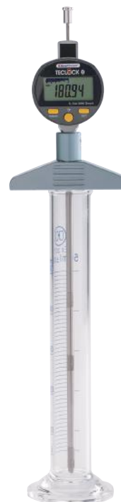
The inner depth is 180.94mm. The length of stylus is extended by the extension rods. Depth Gauge : SSD-214
