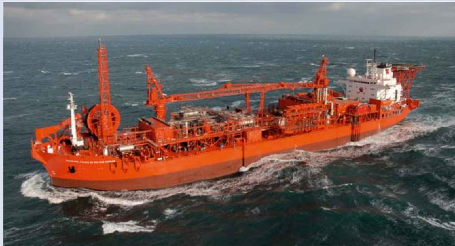
Formerly the 1981-built Aframax tanker Che Guevara , the FPSO Petrojarl Cidade de Rio das Ostras was rebuilt in stages by Norwegian, Polish and Brazilian shipyards for operation in the Siri oilfield off the Brazilian coast. Teekay Collection
