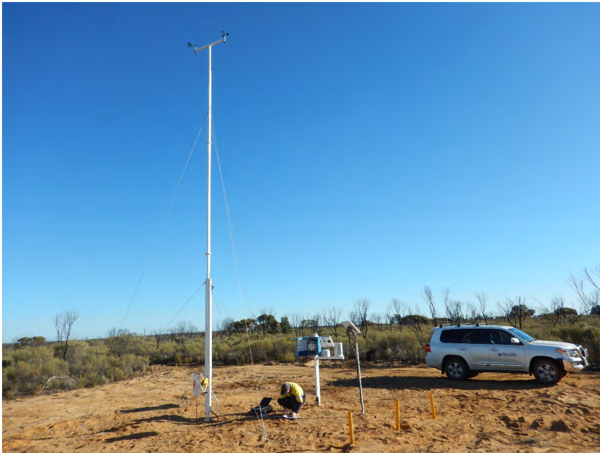
Plate 9-16 The Sandy Ridge automated weather station
