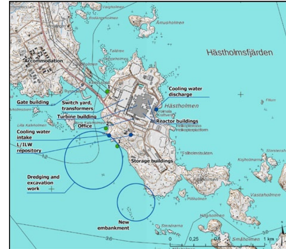
Figure 3-2. The current functions in Loviisa power plant area and the tentative location areas of the planned water engineering measures. The green spots depict the discharge area of the raw water treatment plant (1), the discharge area of the power plant's wastewater treatment plant (2) and the leak water discharge pipe of the L/ILW repository (3).
