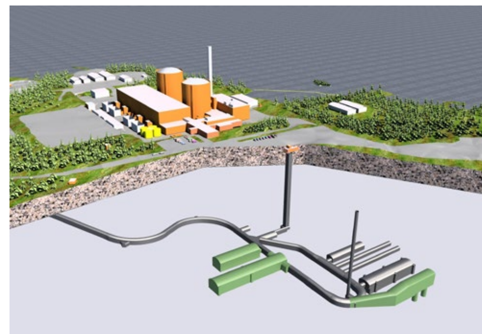
Figure 3-7. An illustration of the final disposal facility of Loviisa power plant for low- and intermediate-level waste. In addition to the existing halls, the illustration depicts the planned final disposal halls for decommissioning waste (dismantling waste halls 1 and 2, a large component hall and reactor vessel silos).
