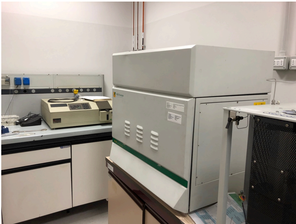
Fig. 2.3.3.b: The isotope Ratio Spectrometer (IRMS) at the ENEA center of Bologna.
