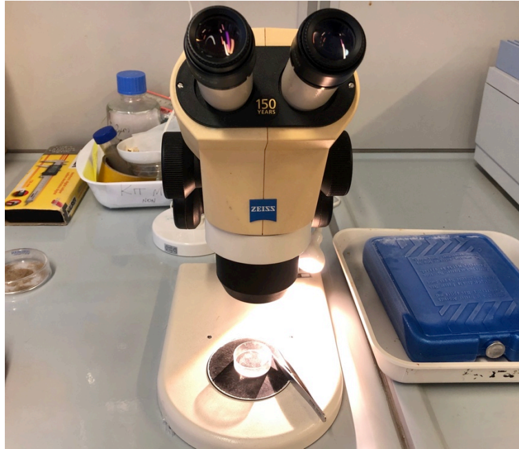
Fig. 2.3: The stereomicroscope used for sorting activity and for animal identification. The ice was used to keep cold sorted animals.
