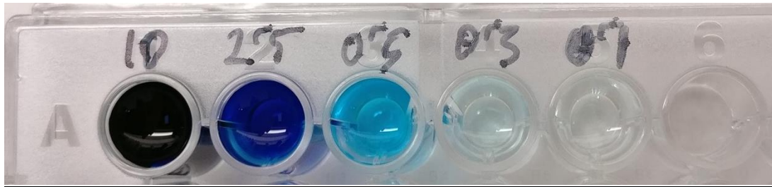
Figura 32: Fotografía mostrando la coloración de diferentes concentraciones de azul de metileno: 10 \mu\text{g}/\text{mL} (31 \mu\text{M} ), 2.5 \mu\text{g}/\text{mL} (7.75 \mu\text{M} ), 0.5 \mu\text{g}/\text{mL} (1.55 \mu\text{M} ), 0.3 \mu\text{g}/\text{mL} (0.93 \mu\text{M} ) y 0.1 \mu\text{g}/\text{mL} (0.31 \mu\text{M} ).
