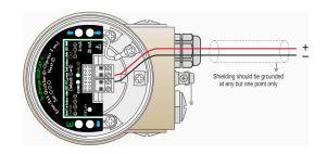
The unit may be damaged by electrostatic discharge (EDS) via its terminal, thus apply the precautions commonly used to avoid electrostatic discharge e.g., by touching a properly grounded point before removing the cover of the enclosure.
