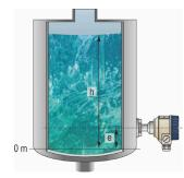
Zero point of the transmitter can also be shifted (offset) outside of the range. This is a virtual extension of the range by adding a dead zone of "e" in which no measurement will take place consequently current output remains the same and the value of "e" will be displayed. The measurement will only be active in the range of "h" however the value of "e" will be added to the level measured.
