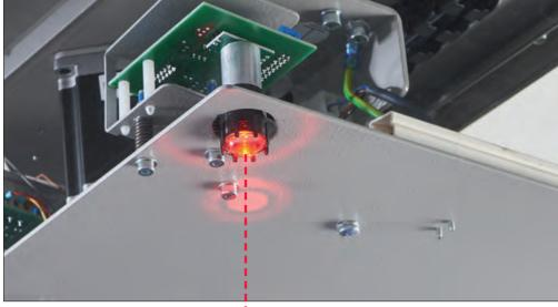
Hänel Pick-o-Light-Vario® moves freely along two axes. An LED unit inside the top of the access point...
