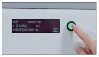
The Hänel digital picking display indicates where the requested item is located in the system and also provides additional information about the item and its storage position
