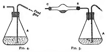
This method is scarcely so sensitive as the preceding one, but has the advantage of removing the sulphuretted hydrogen completely, and a purer coal gas therefore escapes at B, which does not blacken lead acetate paper. We will now pass this purified coal gas, which consists very largely of hydrogen, through a tube containing molten sulphur (BC, Fig. 5).
