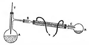
The liquid is poured into A and raised to boiling. The temperature at which the vapour escapes is noted by thermometer T. The vapour passes through the condenser BC, which consists of a tube surrounded by an outer jacket, and kept cool by a current of cold water. The vapour condenses and collects as a liquid in the receiver R.
