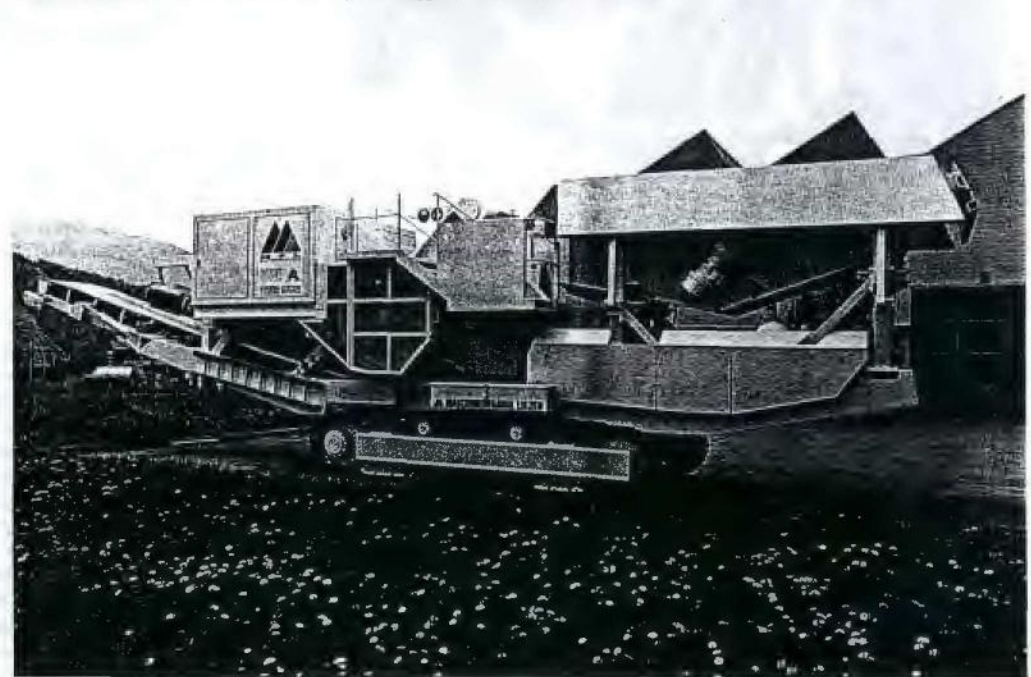
R-CI 108-80/T crawler-mounted recycling with toggle-jaw crusher ▼
