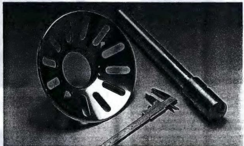
Ignition guard, burner nozzle 534F-2 ▼
