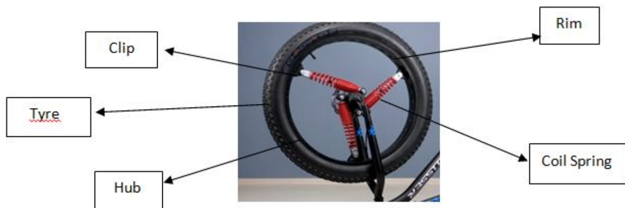
Fig-1: In-Wheel suspension system
