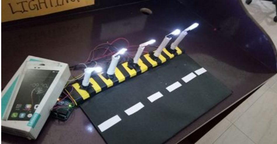
Fig-5: LEDs are ON when LDR is shaded by an object.
