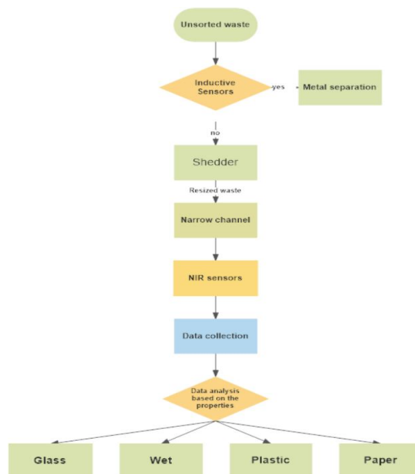
Fig-2: Flowchart showing the operation of waste detection and segregation.
