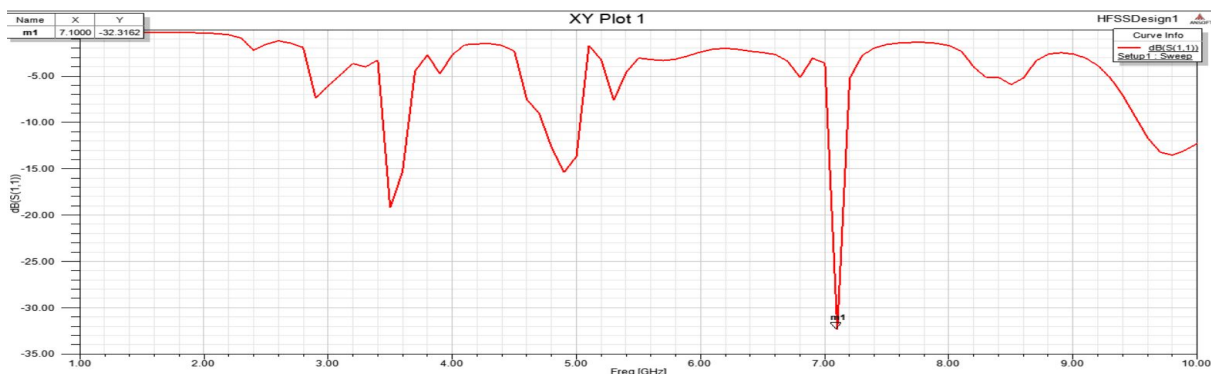
Figure-4: S11 vs. frequency plot for 7.1GHz
