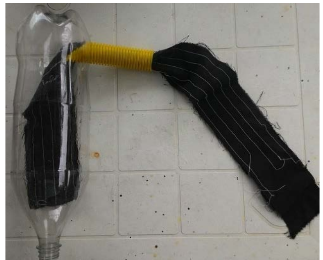
Figure 1: PETI-BR's unit: a 2-litre PET bottle and fabric strips.
