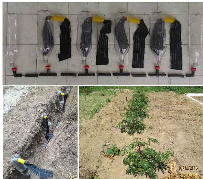
Figure 2: PETI-BR system and installed in a site for cultivating a cassava crop.
