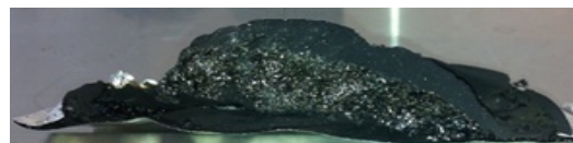
Figure 1: Cross-section of the PA6/GAS2.5%/MPP2.5% formulation at the end of the MLC test.
