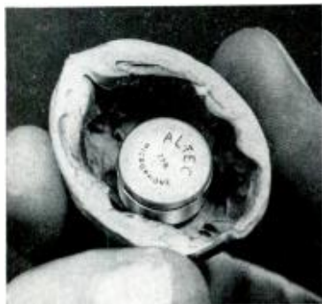
The miniature condenser type microphone, photographed inside a walnut shell, is shown here actual size.
