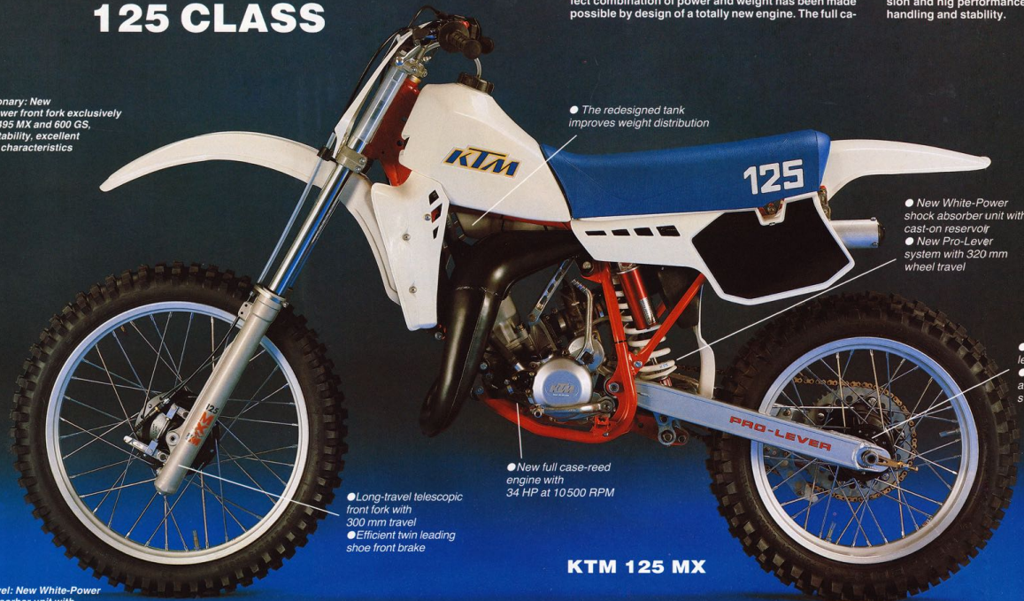
Long travel: New White-Power shock absorber unit with cast-on reservoir. Rebound and compression dampening separately adjustable.
