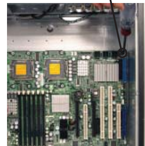
Mounting MB into the Chassis
