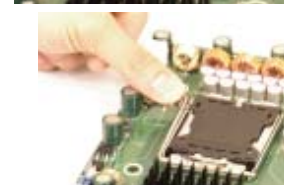
PnP Cap on top of the Load Plate
