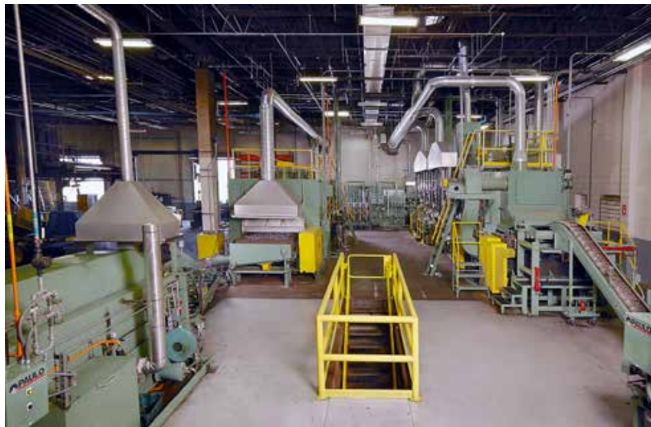
Paulo’s continuous belt furnaces have world-class control systems enabling repeatable quality processing at high volumes.
