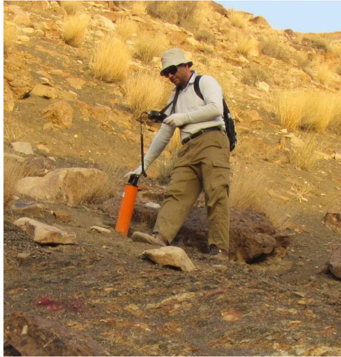
Fig. II.2: Measurement of gamma-ray with GS-512.
