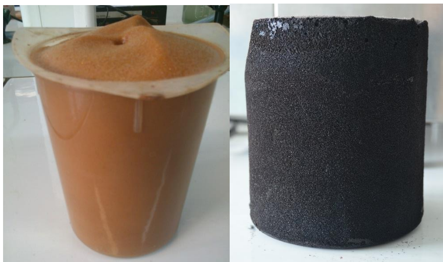
Fig 2. Left. Liquid tannin foam. Right. Rigid tannin foam obtained with the new method.
