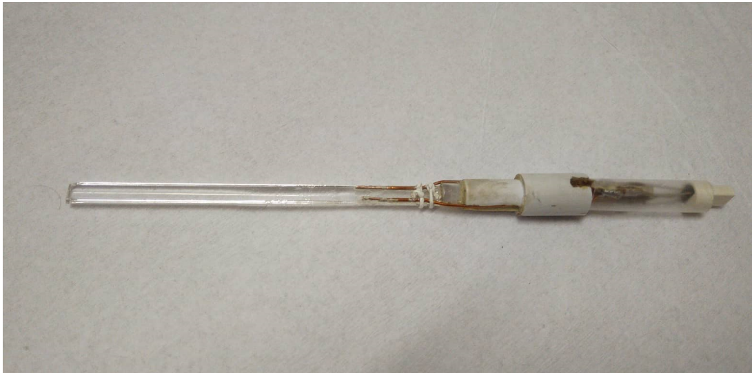
Figure 3.4 – Homemade sample holder adapted for electric measurements.
