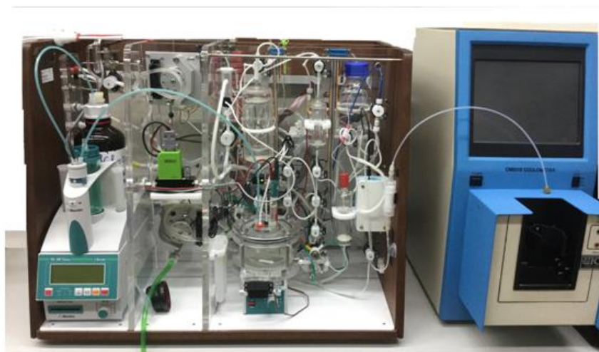
Figure 3-14: Equipment used for the determination of TA and DIC that includes the VINDTA 3C system coupled with a CM5015 coulometer and a 785 DMP Titrino.
