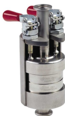
Figure II.1 – Four stage Dekati© cascade impactor used in this study. The stages correspond to, from top to bottom: >10 \mu\text{m} , 2.5-10 \mu\text{m} , 1-2.5 \mu\text{m} and 0.1-1 \mu\text{m} .
