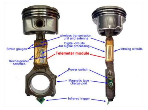
Figure 1.18 Fang telemetry system on a connecting rod [17], [28]
