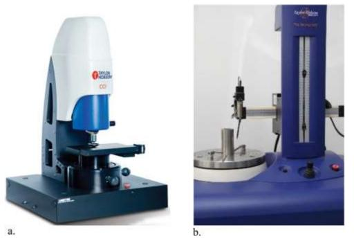
Figure 2.12 Surface topology measurement machines: a.: Talysurf CCI 6000; b. Talyrond 356
