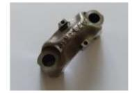
Figure 2.27 Eddy current gap sensors mounts
