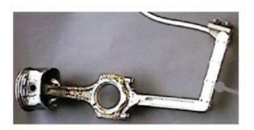
Figure 1.17 Merrit connecting rod grass hopper linkage [26]
