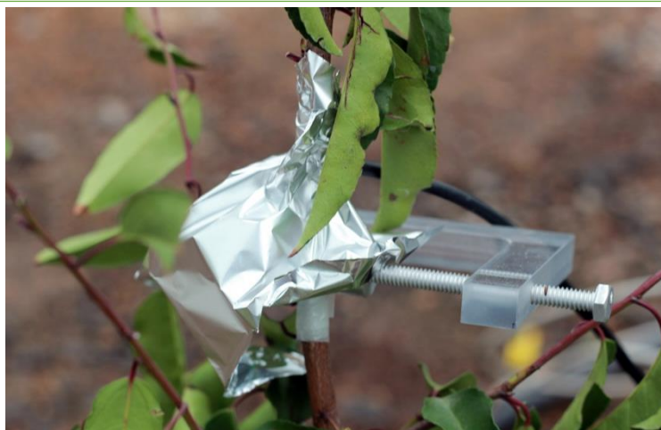
Figure 32. Stem psychrometer installed on a Prunus lusitanica tree, covered in aluminium foil to protect from direct sunlight exposure.
