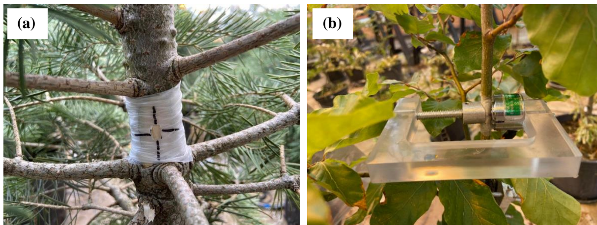
Figure 57. Installation steps of a stem psychrometer.
