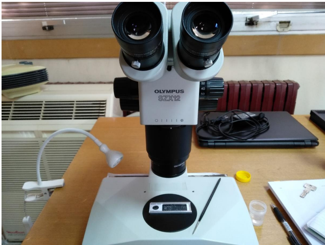
Fig 3.4 Binocular stereoscopic microscope used to analyse the benthic foraminifera (University of Zaragoza, image by Maria Elena Gastaldello).
