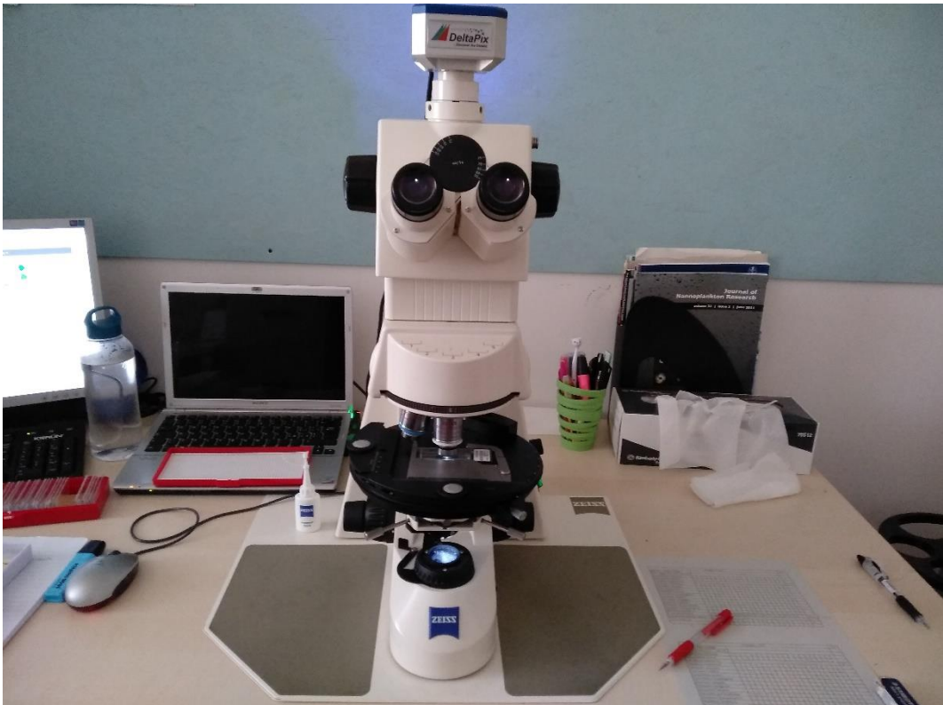
Fig. 3.9 Optical polarizing microscope used to analyse the samples and to take pictures through DeltaPix digital camera and DeltaPix Insight software (image by Maria Elena Gastaldello).
