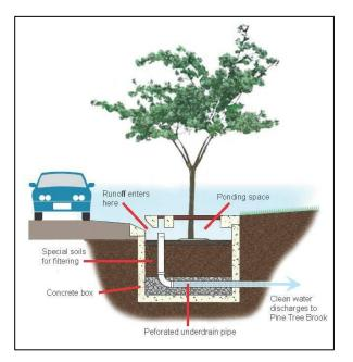
Figure 17: Basic tree filter box diagram Image credit: Town of Milton, MA Dept. of public works stormwater
