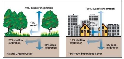
Figure 1: Relationship between impervious surfaces and stormwater runoff.<sup>1</sup>
