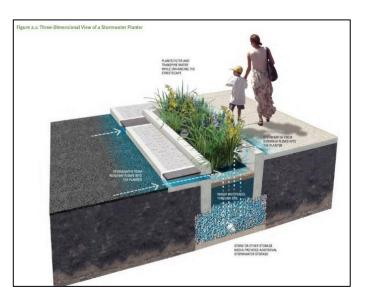
Figure 18: Street-side stormwater planter diagram Image credit: Philly Water
