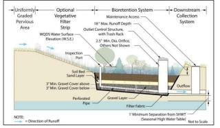
Figure 15: Bioretention facility cross section with underdrains. Image credit: NJ-BMP Manua
