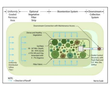
Figure 14: Basic bioretention system design. Image credit: NJ-BMP Manual
