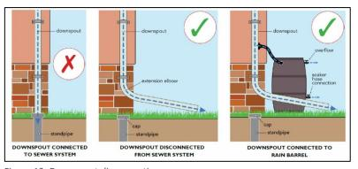
Figure 13: Downspout disconnection Image credit: DC-Water
