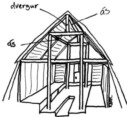
Figure 2. The position of the dvergur (pl.) in the hall (drawn by Karen Bek-Pedersen).
