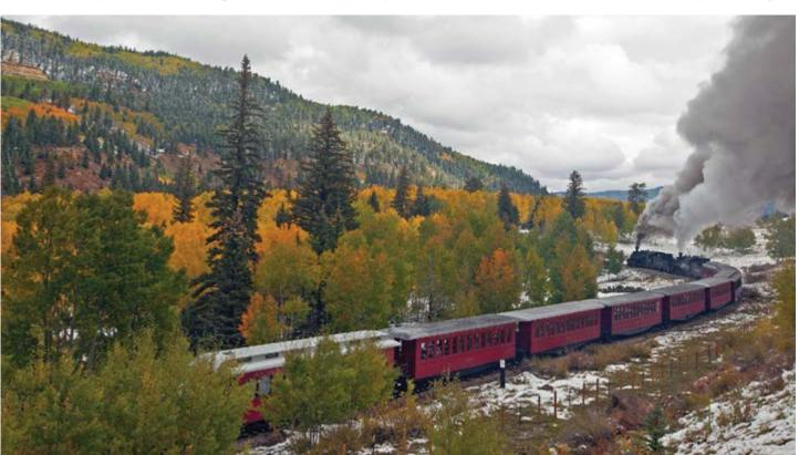
Left: "Doubleheading" Cumbres & Toltec Railroad locomotives enter a sharp curve pulling eight passenger cars over a snow-scattered landscape. Two locomotives are needed when passenger demand requires more cars than usual. A single Baldwin K-36 usually can pull up to six passenger cars.
