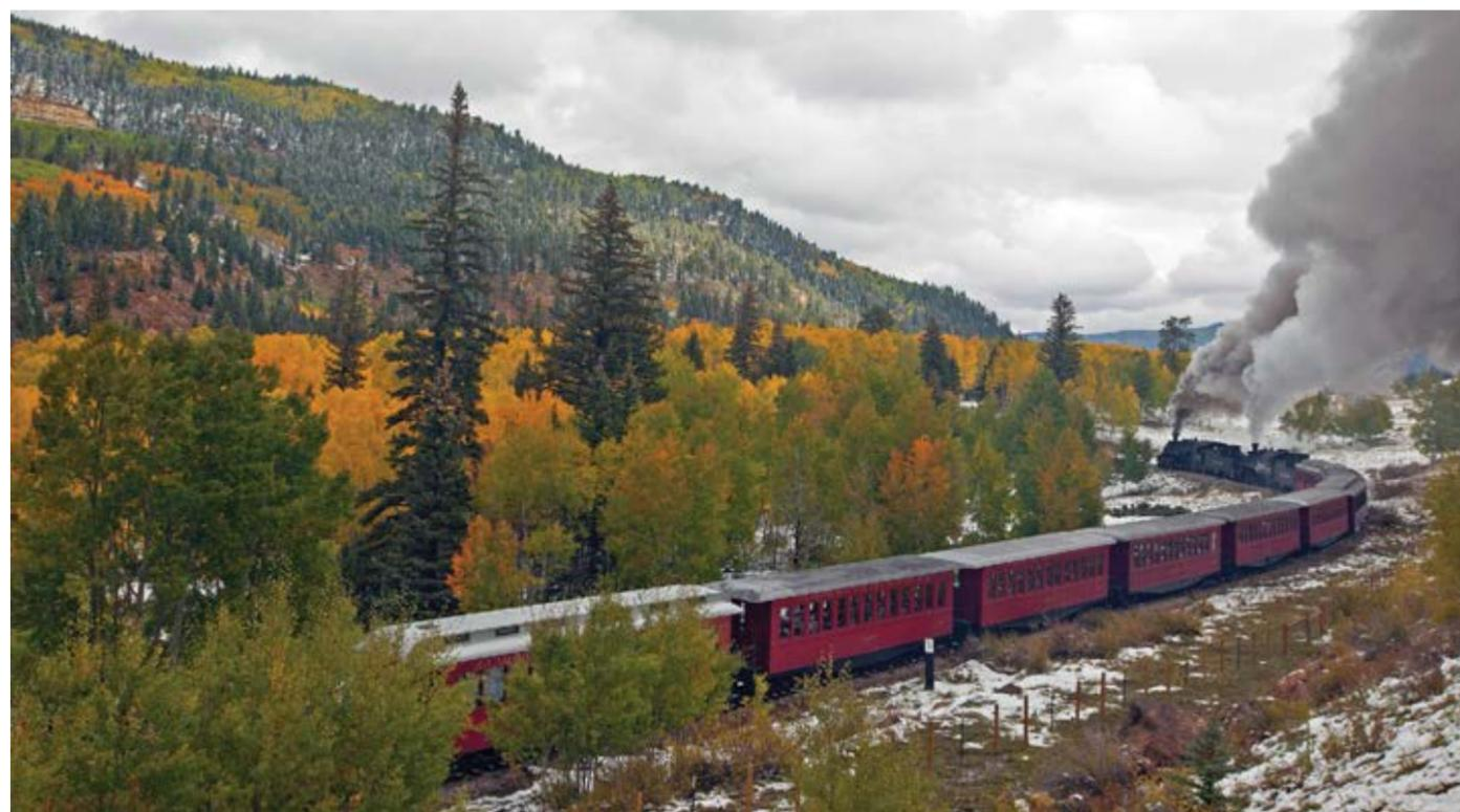
*Left:* "Doubleheading" Cumbres & Toltec Railroad locomotives enter a sharp curve pulling eight passenger cars over a snow-scattered landscape. Two locomotives are needed when passenger demand requires more cars than usual. A single Baldwin K-36 usually can pull up to six passenger cars.
