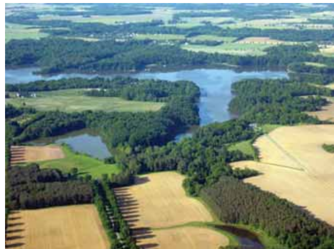
Figure 13. Riparian forest buffer example showing shorelines buffered from farm field by thick stands of trees.
