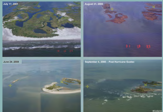
Example: Progressive land-loss of the Chandeleur Barrier islands. The islands are increasingly dissected as the beach is lost, breaching prevails, and marsh lands erode. (Photos: USGS)
