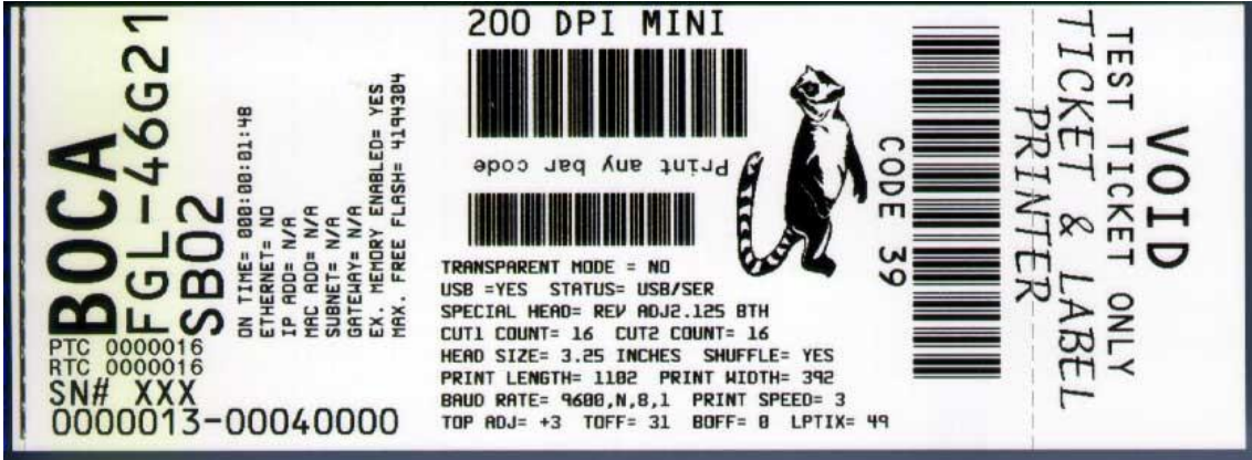
Above sample was printed on a 2" x 5.5" ticket using a 200dpi FGL protocol Lemur with cutter.
