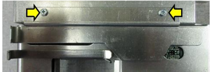
Above is a RADJ2 paper guide w/ load opto
