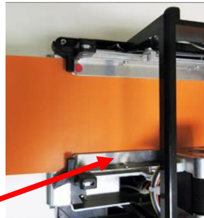
Above shows the UPG adjusted for 3.25" wide media
