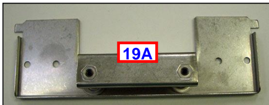
The above head plate is only used on plastic print cage printers and 2003, 3003, 2004 or 3004 print head.
