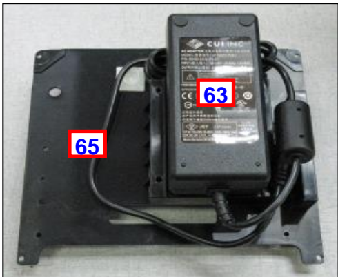
Lemur & Lemur-K printers built after below dates used a 424009-L power pack: June-2016 220VAC S/N 366455 & higher August-2016 110VAC S/N 371579 & higher
