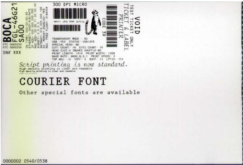
Above sample was printed on a 4" x 6" ticket using a 300dpi FGL protocol Lemur without cutter.
