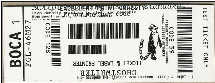
Above sample FGL ticket was printed on a 2" x 5.5" (concert) ticket using a RADJW-2 200dpi FGL printer
