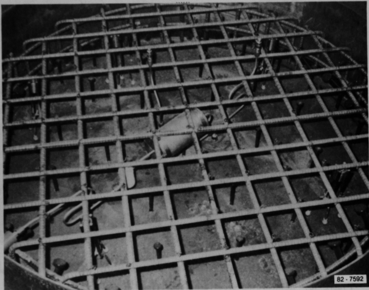
Figure 9. Vent system in the lid of the prototype High-Integrity Container (S/N002).
