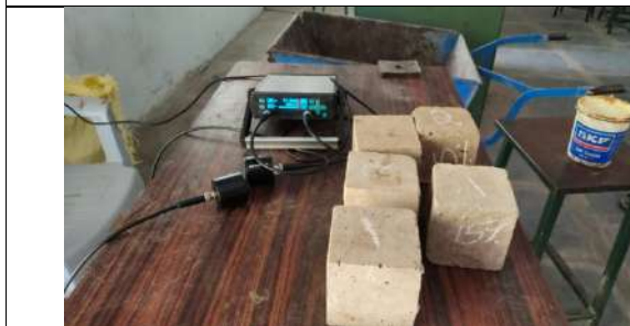
Figure 3: Setup of UPV testing
