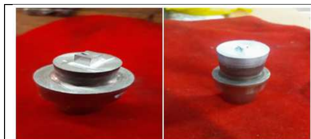
Fig. 1. Square tool pin profile & Triangular tool pin profile
