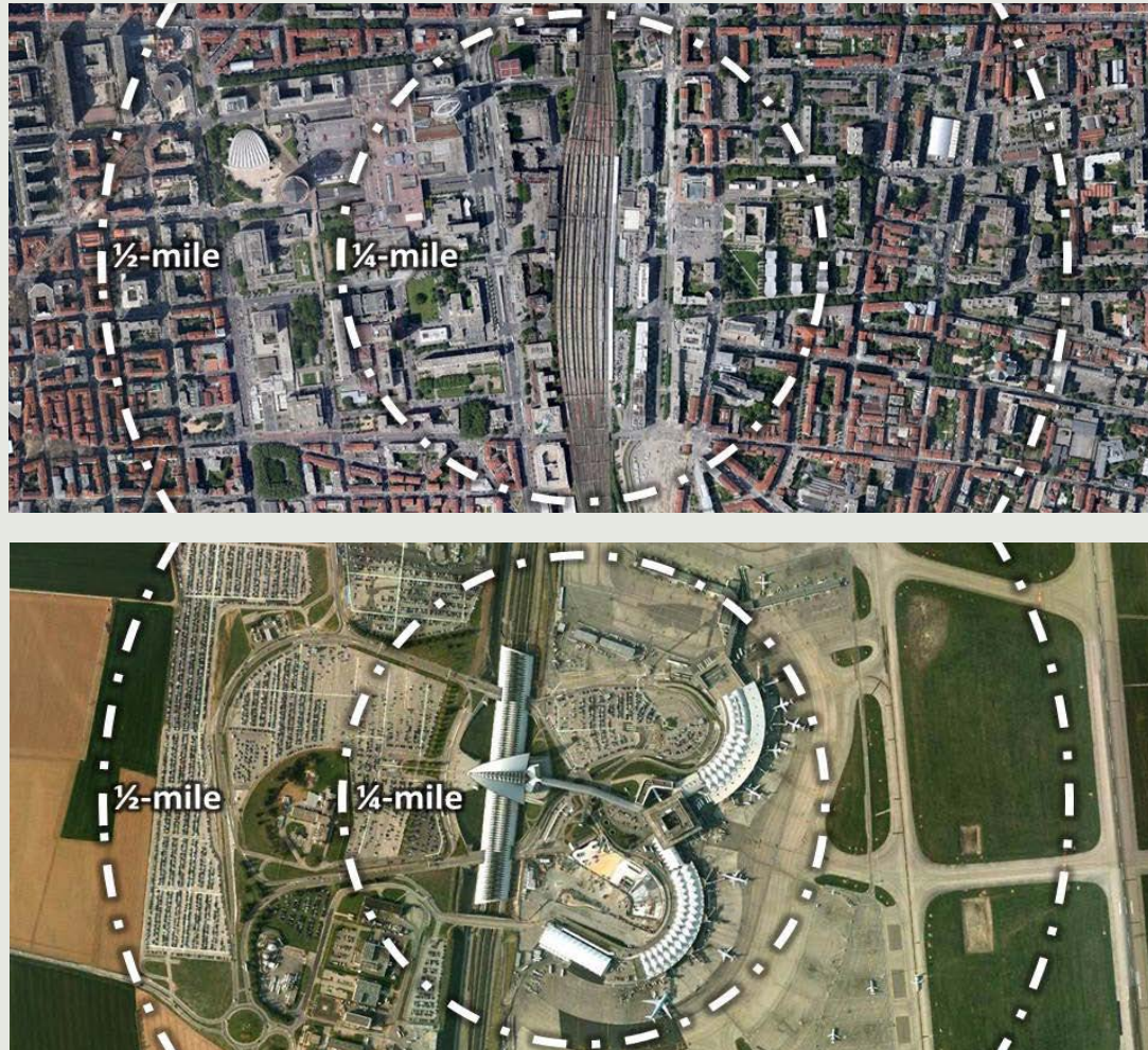
Lyon Part-Dieu, Lyon's main train station (top) shown at the same scale as city's airport, Lyon St.-Exupéry (below), which also includes an HSR station. While Part-Dieu station has a much smaller footprint than St.-Exupéry and is tightly knit into surrounding development, it accommodates over three times as many passengers per year (26 million vs. 8 million).
