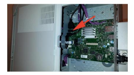
and insert the Bardimm micro USB cable plug stick into that slot, as follows:
