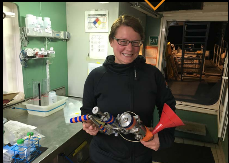
Figure 2. PMEL scientist Tamara Baumberger in the wet lab holding a gas-tight sampler.
