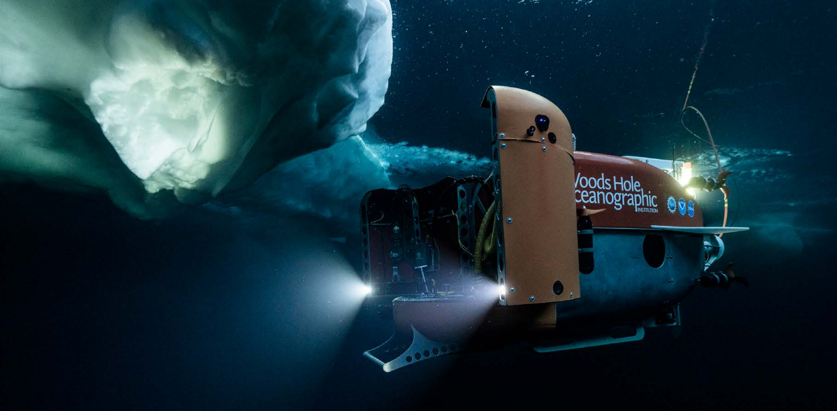
FIGURE 3. The Nereid Hybrid Tethered vehicle shown during a recent NOAA OER-funded expedition to Gakkel Ridge (Arctic Ocean) aboard the Norwegian icebreaker Kron Prins Hakkon is an important component in OECI’s technology development. Image credit: Luis Lamar
