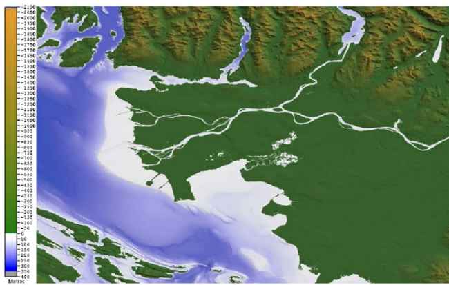
FIGURE 2. Canadian Safety and Security Program 3 m horizontal resolution DEM for the lower mainland, southwest British Columbia.
