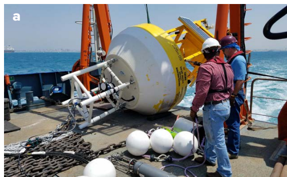
FIGURE 1. (a) A THEMO buoy is prepared for deployment in the eastern Mediterranean Sea off the coast of northern Israel. (b) The THEMO Shallow Buoy is a 2.25 m discus buoy equipped for near-real-time reporting of MetOcean parameters and with downward-looking ADCP.
