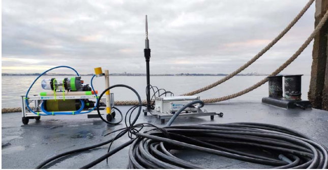
FIGURE 3. The N2ODE prototype is shown ready for deployment near the Troia peninsula south of Lisbon, Portugal.
